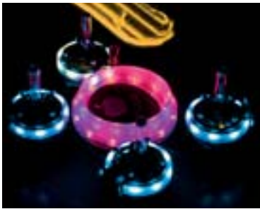
Four robots communicate by blue light that they have found a food source
